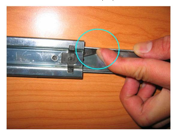
3. Locate the lever on the right hand side and flip it down as shown below
