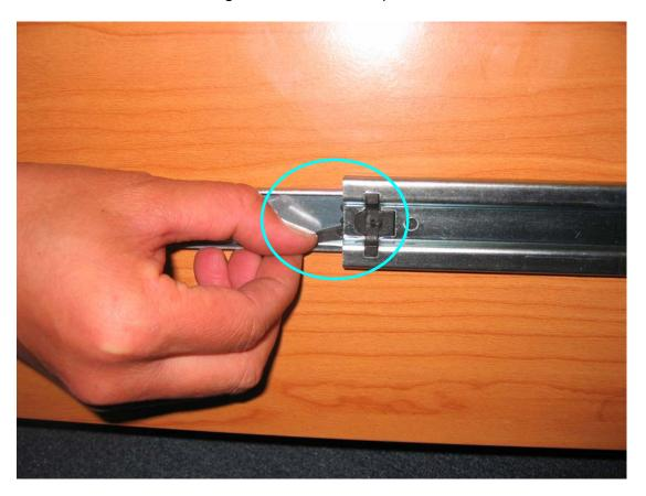
4. Both hands should in the position as below with both levers fliped
